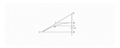
since it was assumed that AB (or BD) is the measure of the time and of the momentum of speed in fall BD from rest at B, then BG will be the time, or measure of time and [of] impetus [in fall BF], at F, coming from [rest at] B [by Proposition III, Theorem III]. If, therefore, BO is taken equal to BG, the added diagonal AO
