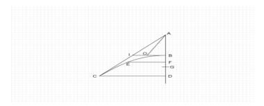
will be the quantity of impetus at point E; for AB is assumed to determine the time and impetus at B, which (impetus) turned through the horizontal continues always the same, while BO determines the impetus at F (or E) through fall from rest at B through altitude BF. But AO is equal in the square to both AB and BO together [by Proposition II. Theorem II.,  $AO^2 = AB^2 + BO^2$ ]; what was sought is therefore evident.
