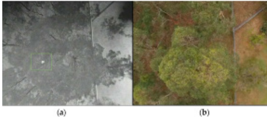
Figure 1. This shows the difference in greyscale imaging using thermal (a) and standard digital view (b). (Gonzalez et al. 13)
