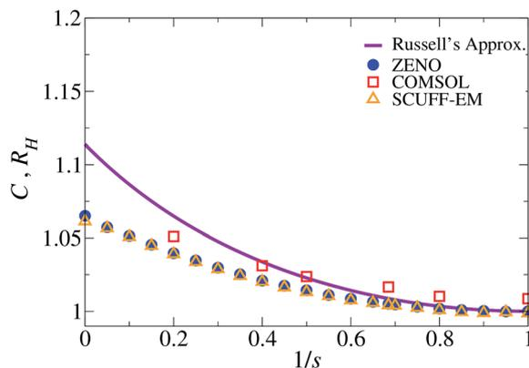
Fig. 2 Self-capacitance  $C$  and hydrodynamic radius  $R_h$  for cube-like particles. Values are normalized such that all particles have the same volume as a sphere with radius one. Russell approximation<sup>53</sup> is equivalent to a spherical harmonic expansion to first order and is discussed in Appendix B.
