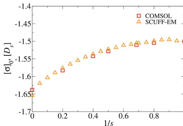
Fig. 4 Intrinsic conductivity of a perfect insulator  $[\sigma]_0$  and the intrinsic solvent diffusivity  $[D_s]$  for cube-like particles.
