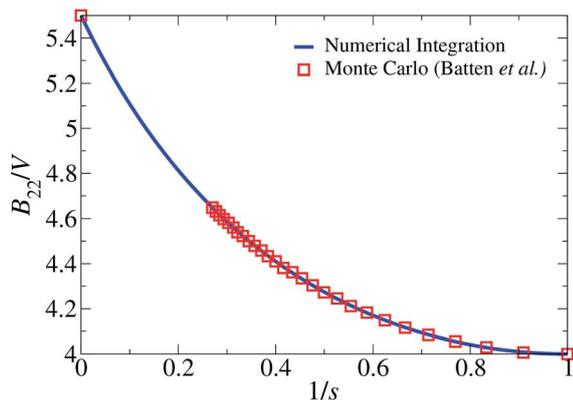
Fig. 5 Second osmotic virial coefficient  $B_{22}$  normalized by volume for cube-like particles. Symbols correspond to quantities calculated by Batten *et al.*<sup>23</sup> using a Monte Carlo method.
